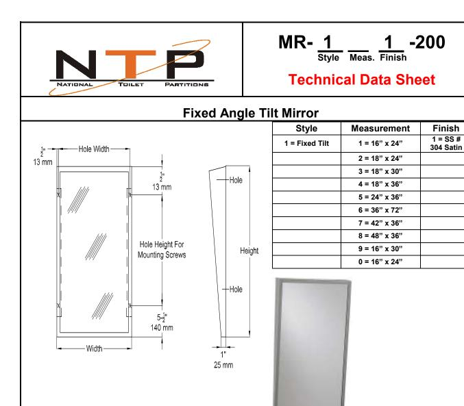
**MATERIALS:** The fixed angle tilt mirror is fabricated of alloy 18-8 stainless steel, type 304, 20 gauge, No. 4 satin finish.
